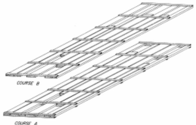
Fig. 1. Proper placement of random length boards in successive layers.
