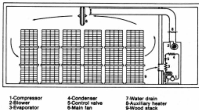
Fig. 3. View of a typical dehumidification kiln.
