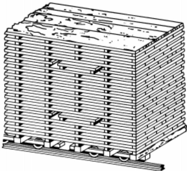
Fig. 2. Lumber stacked for kiln drying showing location of kiln samples
